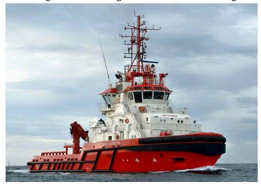
AHT / Azimuth Stern Drive Main engines: 2 x ABC 8DZC, 2 x ABC 6DZC
